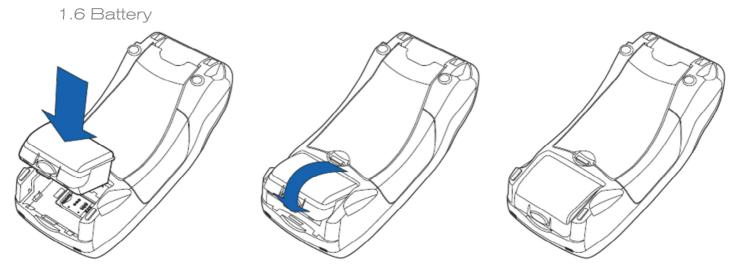
The battery is attached by placing it on its slot and pressing it downwards.
