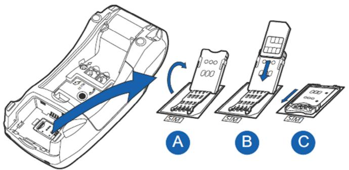
The SIM-card is placed beneath the battery so that the chip is facing down and the folded corner points downwards.
