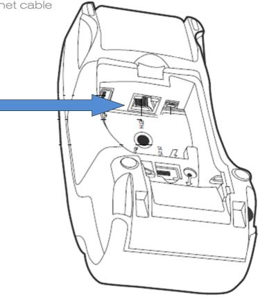
Connect the ethernet cable to the ETH-port at the bottom of the terminal. The other end of the cable is connected either to a broadband modem or plug.
