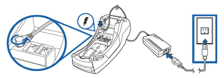
Connect the adapter to the main power cord, the power cord to the power supply and the plug to the electrical outlet. The adapter is connected at the bottom of the terminal into the left port.
