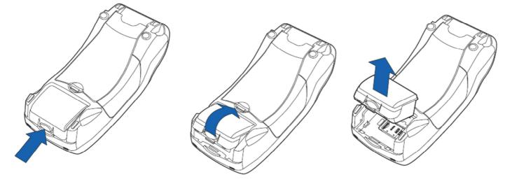
To remove the battery, press the locking tab and pull the battery from its slot.
